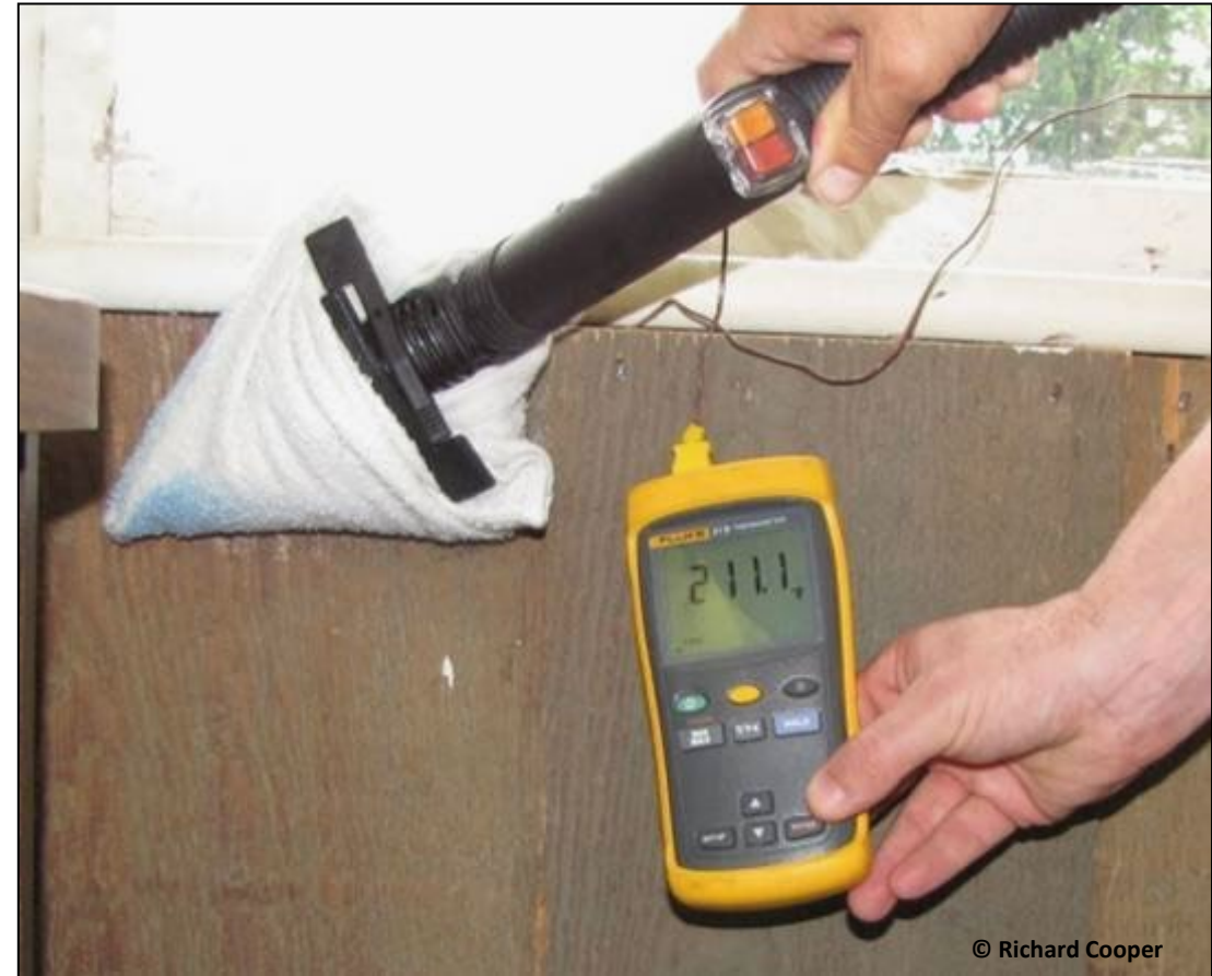
Window Frame ¼" Wood Panel 211.1°F (99.5°C)
